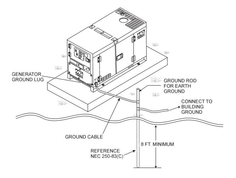
Figure 4. Typical Generator Grounding Application
